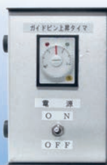
手動用制御 Box (磁気センサー付き) Manual Control Box (with magnetic sensor)
